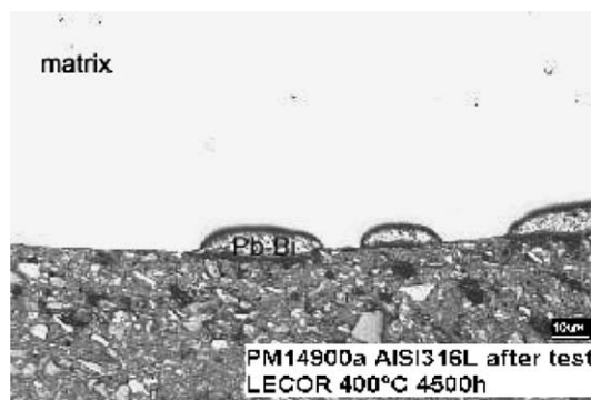
Fig. 2. Optical micrograph of austenitic steel exposed in LECOR loop after 4500 h ( C_{[\text{O}_2]} = 10^{-8} – 10^{-10} wt%, T = 400 °C).
